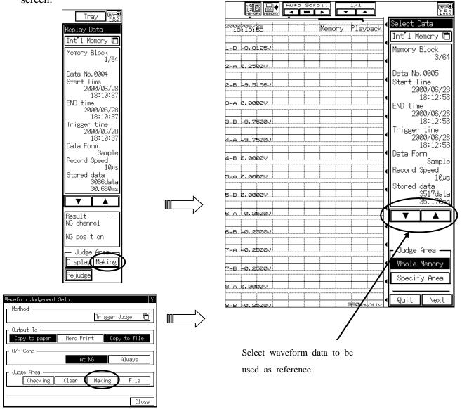
If the entire memory block is to be used for waveform detection, select (Whole Memory), if only a portion is to be used, select (Designate range).
