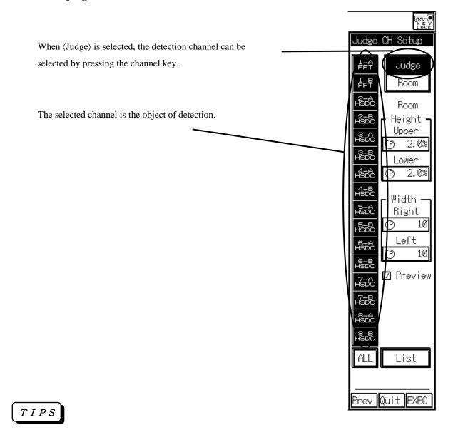
On the reference waveform, only the channel actually compiling data can be selected.
